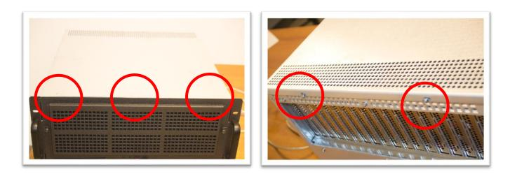
With the unit open, remove the chassis card hold-down bracket located over the SHBs and secured with 4 screws, 2 each on either side of the unit and remove from the system.
