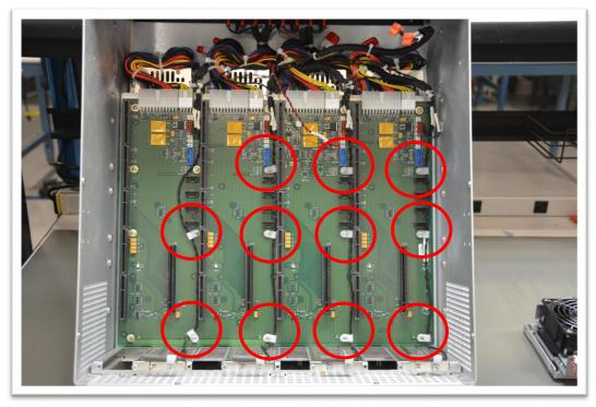
Using four 6-32  $\frac{3}{4}$ " screws, and 1/4" cable clamps, secure the body of the temperature probes to an I/O bracket screw hole, as indicated.
