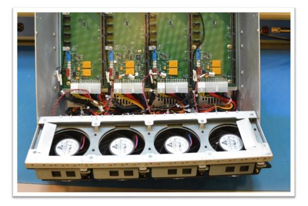
Orient as it will be installed in the system and install the Fan Fail Connector to the Fan Fail port on the FSC1401.
