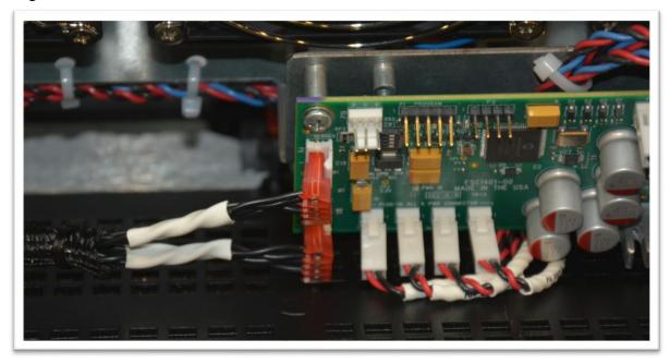
Insert the fan bar into the operational position and confirm that all wires are properly secured. Reinstall the fan bar using the screws that secured it previously.
